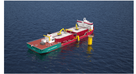
A rendering of the Great Lakes' new subsea rock installation vessel for the offshore wind market.
